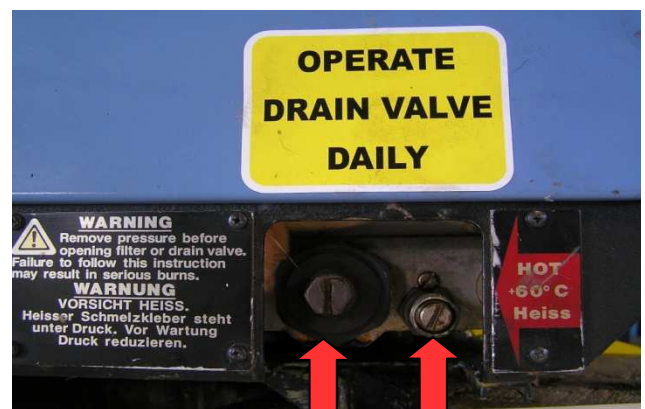
TANK FILTER DRAIN VALVE
